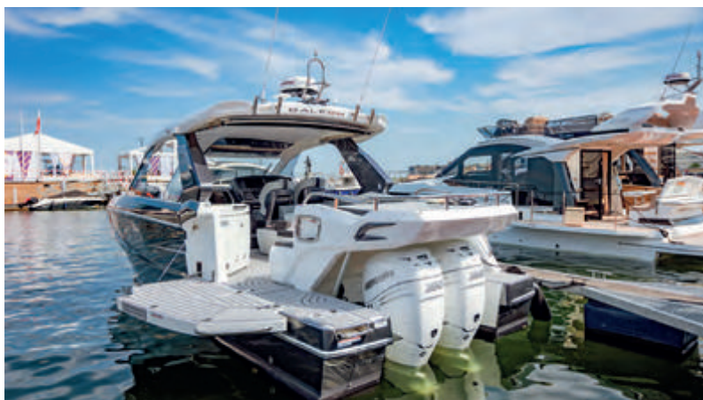
Galeon's 325 GTO (left) with twin 350hp Mercury outboards; the 375 GTO (right) with two 600hp Mercury V12 Verado engines
